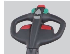
Tiller All operating elements on the CAN tiller are easy to reach.
