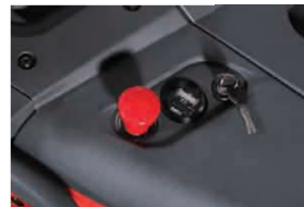
Key-switch, emergency switch and battery discharge indicator.
